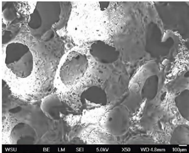
Interconnecting pore structure contains nano to micron pores
